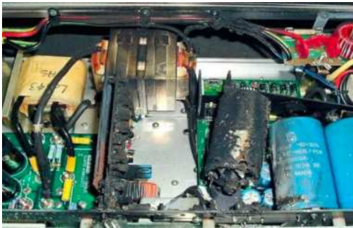
PCB Failures due to high harmonics
